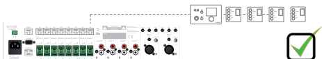
Multiple wall panels (only one with audio input) on one WP port
